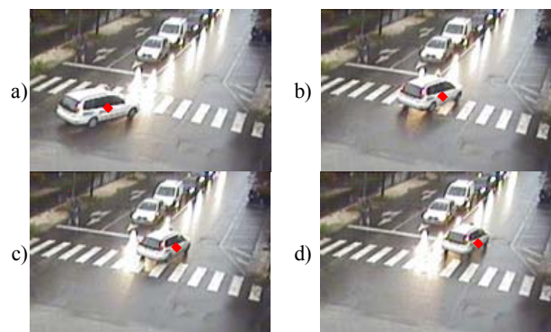
Figure 4: the tracked car along with the found reference point (red star) using the maximum absolute strategy. The reference point is in the same position of the car: a)frame #230, b)frame #238, c)frame #243, d)frame #246
