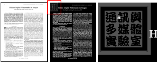
Fig. 9 A digital document marked with the proposed scheme and the extracted result out of the inverted version. Enlarged view of the marked area is also listed.
