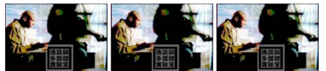
Fig. 8 Gamma-corrected frames out of a H.264 video sequence compressed using different QP values (QP=6, 12 and 18) respectively.
