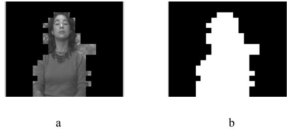
Fig. 3. result of block-based segmentation (silent sequence) (a) region of object in original image (b) binary mask
