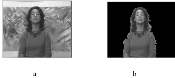
Fig. 6. video object in video sequence. (a) a frame in video sequence. (b) automatic VOP extraction results.
