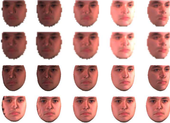
Fig. 3. Results on Synthetic video with Ground Truth Poses. The first row shows the original LR frames and the second row shows the bicubic interpolated ones. Reconstructed SR images are shown in the third row. The last row shows pose and illumination normalized reconstructed SR images with respect to the middle input LR image.
