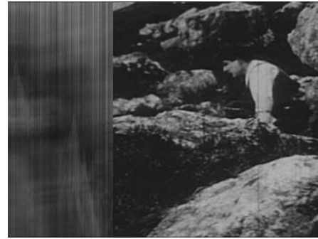
Fig. 3. On the left is a set of horizontally projected slices of 200 images in an archive sequence, one image of which is shown on the right. The presence of flicker and shake can be diagnosed from the varying brightness and the jagged edges of features of the slices as they evolve in time.
