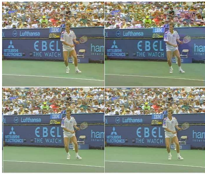
Fig. 7 – Transcoded, decrypted frames: plaintext (top left), sign encrypted (top right), inter-frame transcoder + plaintext (bottom left), inter-frame transcoder + sign encrypted (bottom right)
