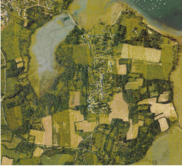
Fig. 2. Projection of classified ground lidar points (brown points) onto an ortho-rectified image.
