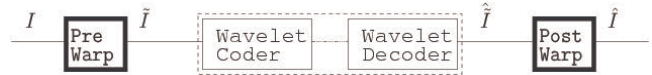
Fig. 1. Goal of the scheme: Pre-Warp the Image so as to adapt the resulting signal to any conventional wavelet coder. Warping parameters are transmitted independently.
