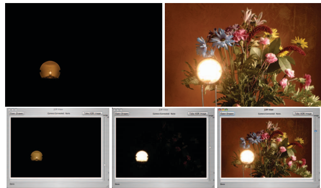
Fig. 1: The top row shows two low dynamic range images taken at both short and long exposure times. The two low dynamic range images are composited to produce a single high dynamic range image. Notice that in the short exposure time image (top left), the shape of the bulb is evident, the position of the filament, etc. However, much of the information of the scene is lost. For example, the flowers to the right of the halogen light are not seen. Conversely, if we look at the long exposure time image (top right), the flowers are present, however, much of the information of the bulb is lost. The bottom row shows a single high dynamic range image in a simple image viewing program. The bottom left image shows the HDR at a gain approximately equal to the input image shown at the top right, and the bottom right image shows the HDR image at a gain approximately equal to the input image shown at the top left. The bottom center image is the high dynamic range image at an intermediate gain, in effect producing an interpolated exposure. Note that the bottom row depicts a single HDR image shown at three different gains. The spatial resolution of the input images is 1520 \times 1007 and uses three color channels (red, green, and blue) which results in a floating point image size of 17.5Mb using IEEE single precision floating point representation.
