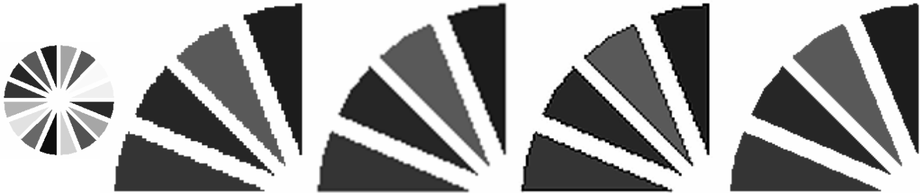
(a) Scaling from 180 \times 180 to 300 \times 300 . From left to right: source image, nearest-neighbor, bi-cubic, bi-cubic+hi-boost, and inter-/extra-polation.
