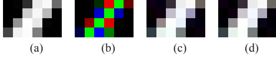
Fig. 2. (a) Original image, (b) CFA samples, and the results of performing high-frequency substitution in (c) wavelet domain, and (d) spatial domain
