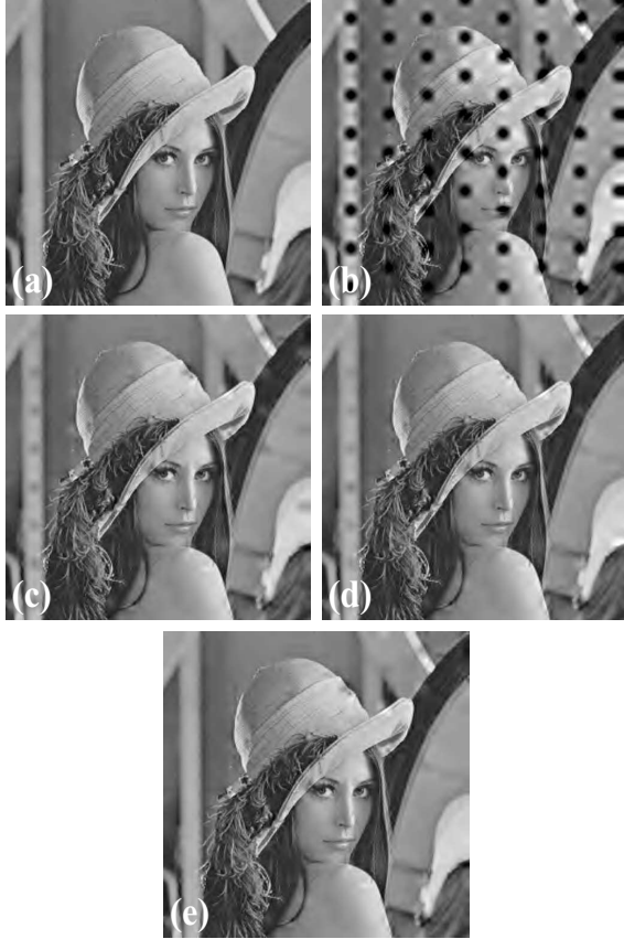
Fig. 2. (a) Lena compressed at 0.208 bpp (PSNR = 32.18 dB). (b) Lena after loss of packet 12. (c) Bilinear interpolation (PSNR = 28.29 dB). (d) MAP approach of [5] (PSNR = 28.54 dB). (e) The proposed method (PSNR = 28.77 dB).
