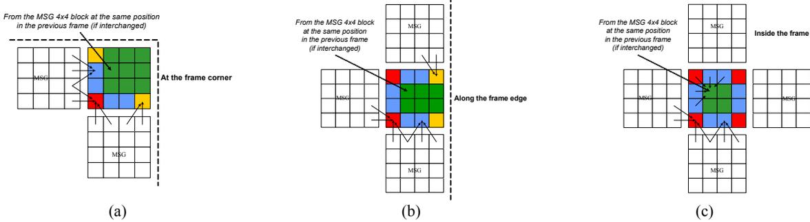
Fig. 4. For STPMV, three types of macroblocks are defined in SSG: (a) corner MB, (b) edge MB, and (c) central MB.
