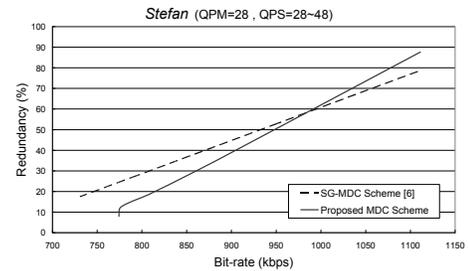
Fig. 7. The redundancy vs. bit-rate curve of *Stefan* sequence.
