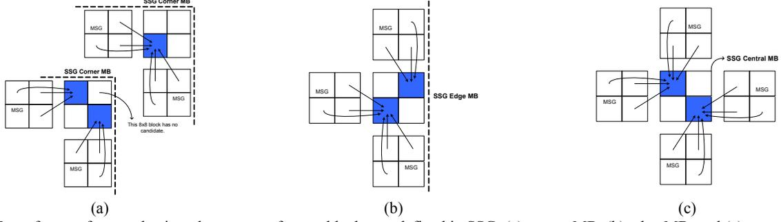
Fig. 5. For reference frame selection, three types of macroblocks are defined in SSG: (a) corner MB, (b) edge MB, and (c) central MB.
