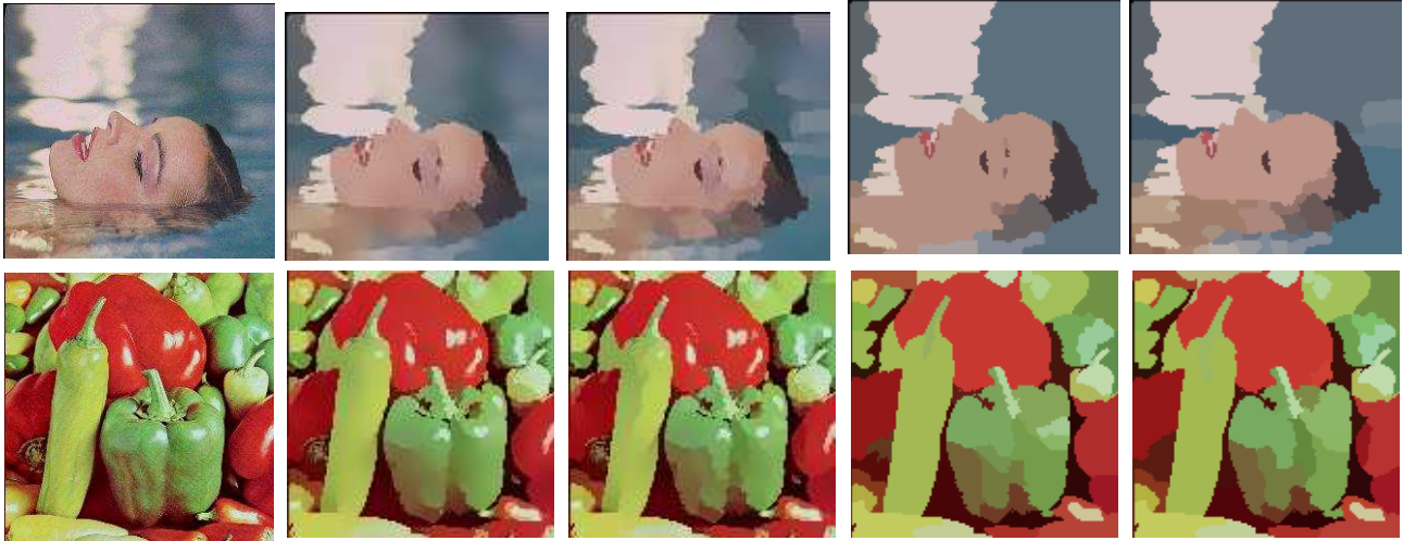
Fig. 1. Filtered and segmented images generated by both the proposed method and the standard mean shift for images: Lady and Pepper. From left to right: original, filtered image using the proposed method, filtered image using the mean-shift filter, segmented image using the proposed method and segmented using the standard mean shift.
