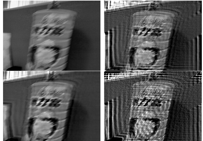
Fig. 5. Top left: blurred image, Top right: restored image by using the regularization-based image restoration method with the initial blur parameter values. The image quality score is 71.3. Bottom left: restored image after the proposed iterative parameter adjustment process. The converged image quality score is 97. Bottom right: result from the Matlab deconvolution function.
