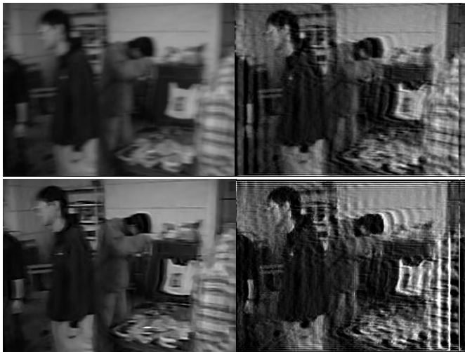
Fig. 4. Top left: blurred image, Top right: restored image by using the regularization-based image restoration method with the initial blur parameter values. The image quality score is 33.2. Bottom left: restored image after the proposed iterative parameter adjustment process. The converged image quality score: 73.5. Bottom right: result from the Matlab blind deconvolution function.
