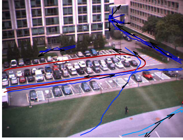
Fig. 3. Typical tracks from the top 20 most significant clusters. Arrows indicate velocity; color shows average size along track (warmer color indicates larger size).
