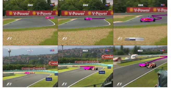
Fig. 3. Images from video shots acquired by two different cameras at two different places on the circuit. The computed trajectories are overprinted on the images.
