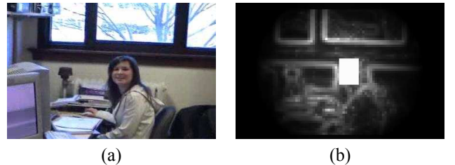
Fig. 4. Highlighting face areas in the saliency map. (a) Original frame and (b) final saliency map.
