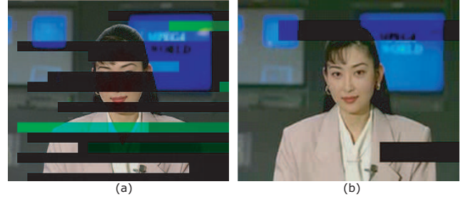
Fig. 5. The reconstructed frames, (a) no loading ratio control (b) loading ratio control when an MS is located at the cell boundary (the normalized distance of 0.95).
