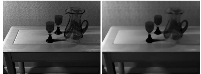
Fig. 1. Median filtering, with a kernel radius of 32, performed on a 6.4 megapixel image in less than one second using our algorithm.
