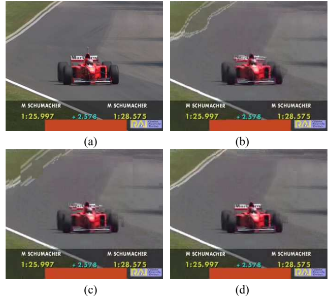
Fig. 4. The interpolated results of frame 56 of FORMULA 1 sequence using (a) original frame, (b) MV smoothing (PSNR: 29.46dB), (c) vector median filtering (PSNR: 29.80dB), and (d) the proposed method (PSNR: 31.56dB), respectively.
