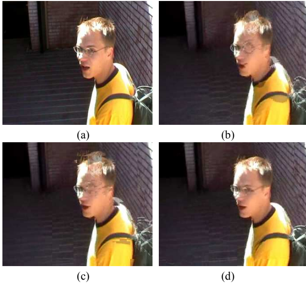
Fig. 3. The interpolated results of frame 288 of WALK sequence using (a) original frame, (b) MV smoothing (PSNR: 19.76dB), (c) vector median filtering (PSNR: 19.67dB), and (d) the proposed method (PSNR: 21.33dB), respectively.
