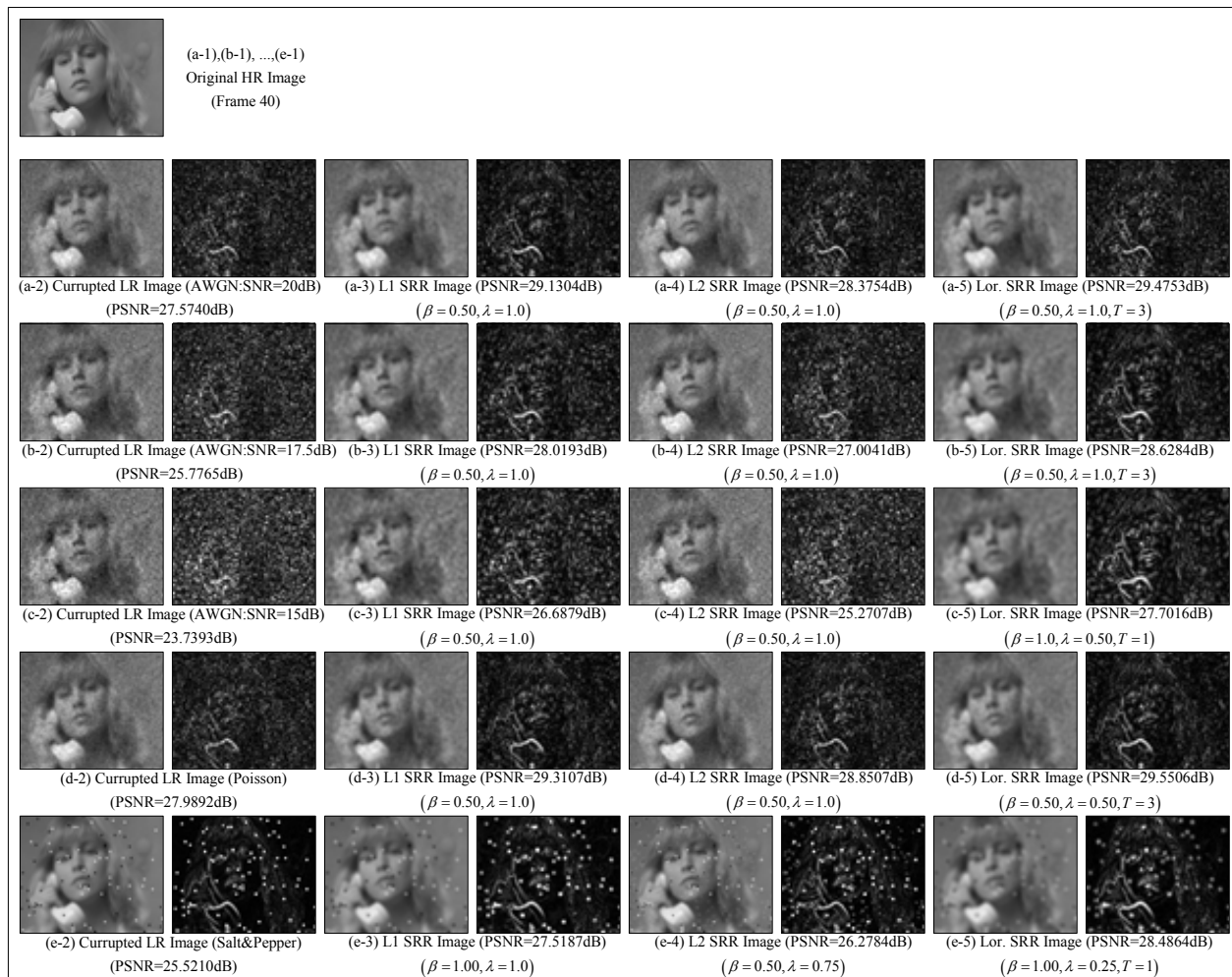
Fig. 1: The Experimental Result of Proposed Method (The right image on our experiment result of each subfigure is the absolute difference between it's correspond left image to the original HR image. The difference is magnified by 5.)
