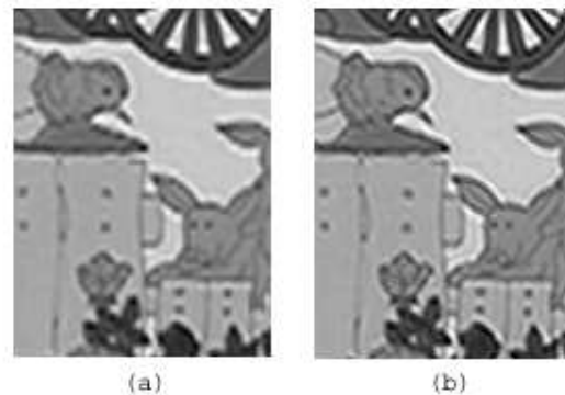
Fig. 8. Results on Calender sequence; (a) bicubic interpolation, and (b) our superresolution result.
