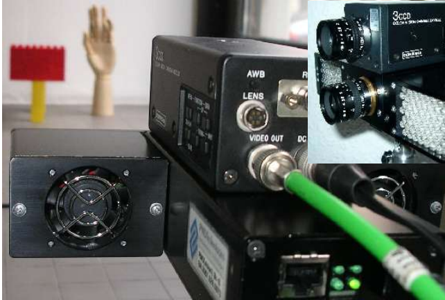
Fig. 2. Piggyback assembly of PMD and color CCD.
