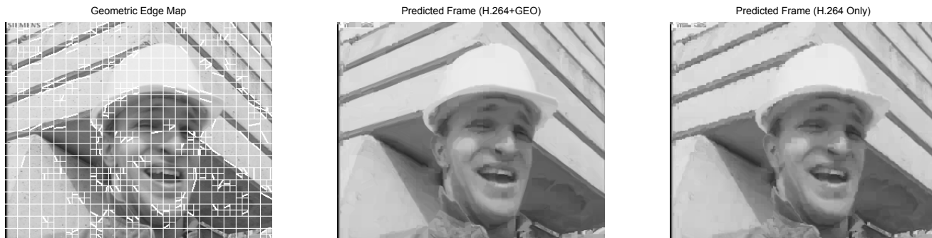
Fig. 5. Experiment with the 15th frame of Foreman(CIF) at QP=28. Left: Intra geometric block partitioning edge map. Center: Intra Prediction (coded residual subtracted) by geometry extended H.264/AVC. Right: Intra Prediction (coded residual subtracted) by H.264/AVC.
