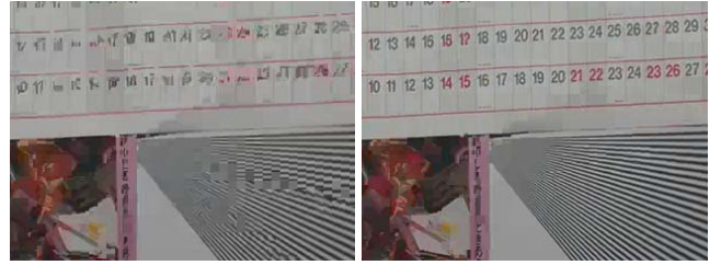
Fig. 5. Example for the prediction signal of H.264 (left) and H.264+ETP (right) for SPINCALENDAR 4CIF at QP=32.
