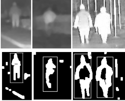
Fig. 2. Dual Adaptive Thresholds segmentation results. The above are original gray-scale images. The below show the segmentation results.
