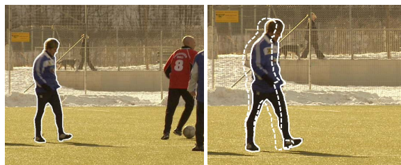
Fig. 7. Tracking on sequence Soccer . The left figure shows the initial, hand-edited contour C_1 on frame F_1 . The right figure shows the computed contour C_5 on frame F_5 (solid line) with C_1 superimposed (dashed line).
