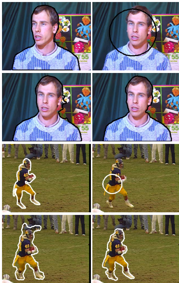
Fig. 1. Segmentation on sequence ‘‘Erik’’, resp. ‘‘Football’’, on frame 6, resp. 75: (from left to right and top to bottom) region of interest \Omega_R manually segmented on frame 1, resp. 74; initialization of the segmentation; result \Omega_T of segmentation with method kNN-KL; result \Omega_T of segmentation with method kNN-KL-G.
