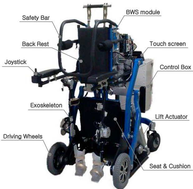
Figure 2. Prototype of the wheelchair integrated lower limb exercise/rehabilitation system
