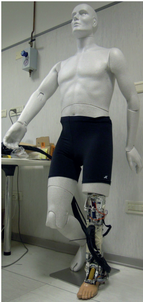
Fig. 13: Completely assembled prosthesis on mannequin.
