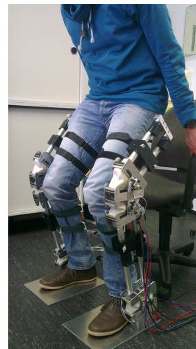
Fig. 5. Exoskeleton robot as testbed for analyzing human robot interaction strategies for lower extremities movements equipped with recently developed soft-actuators.
