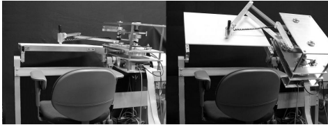
Fig. 11. Quasi-3D mechanism of Neo-PLEMO
