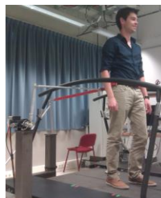
Fig. 1: Experimental setup, used to support lateral balance during walking. It comprises an admittance controlled servomotor, connected to the pelvis via 2 perpendicular rods and a spherical gimbal.
