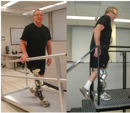
Fig. 2. Transfemoral amputee using the powered knee and ankle prosthesis to ascend a ramp (left) and stairs (right).
