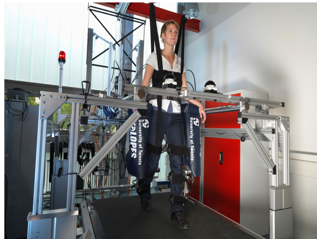
Fig. 1: The Lopes is a bilateral exoskeleton with eight degrees of freedom. The actuators are detached from the exoskeleton and connected to the joints via Bowden cables and springs. The robot is impedance controlled via series elastic actuation.
