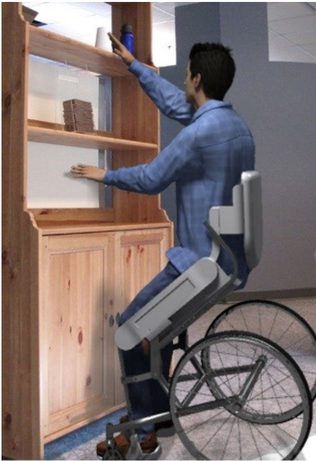
Fig. 1. A user in the COMBO device using the dynamic seating functions.
