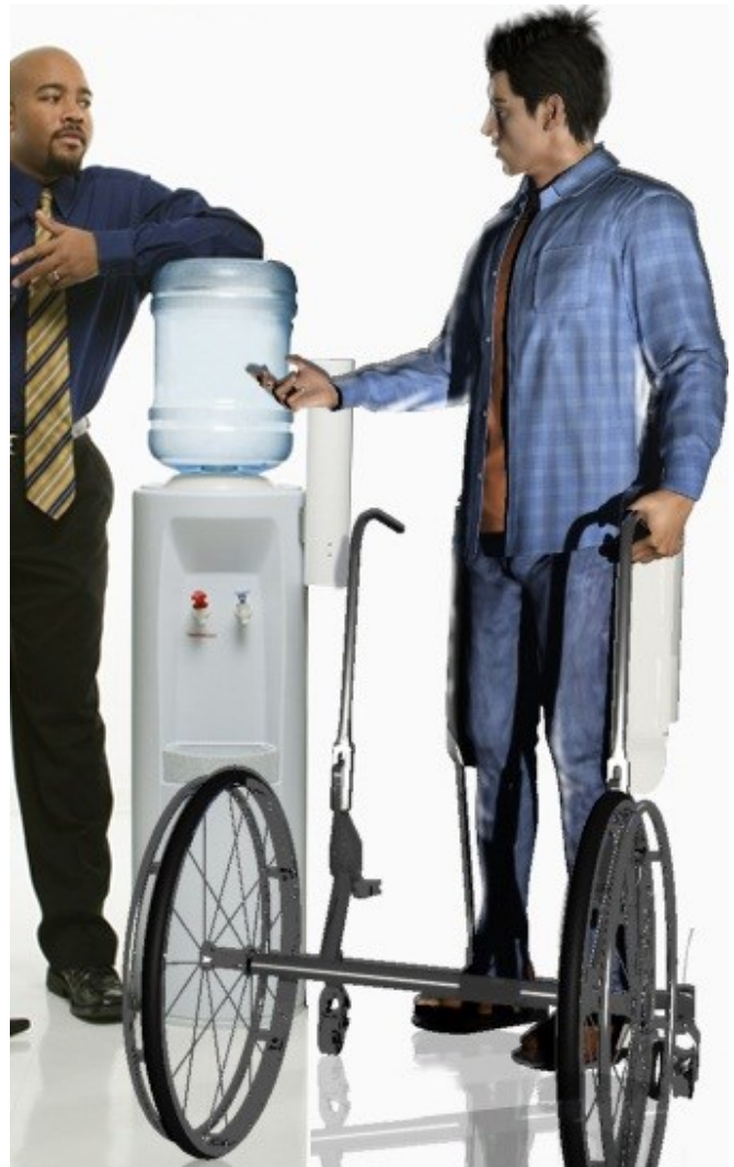
Fig. 2. The COMBO device being used as a walking exoskeleton, with the wheeled frame deployed as a walker for stability. Note: straps (needed for secure attachment to the exoskeleton when standing) are not shown.
