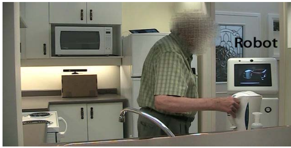
Fig. 2. The robot showing a video prompt to an OAwD during the tea-making ADL
