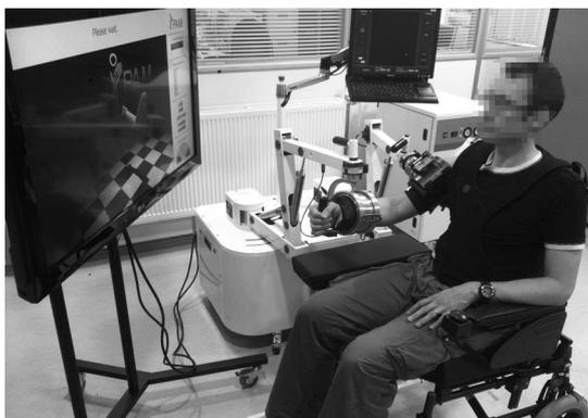
Fig. 2. The iPAM MkII Robotic Rehabilitation System
