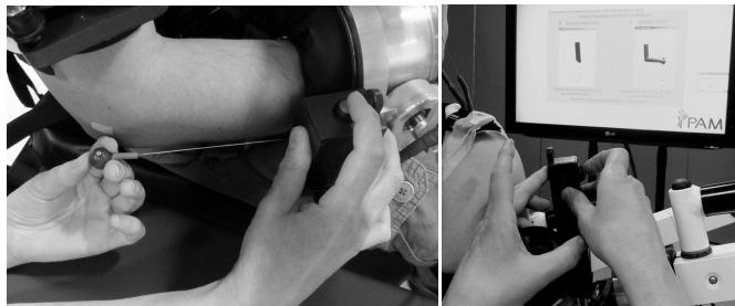
Fig. 4. Calibration tool 1 measuring relative position from lower orthosis to medial epicondyle and calibration tool 2 measuring upper arm angles and comparing patient arm to the human arm model on the Patient Interface.
