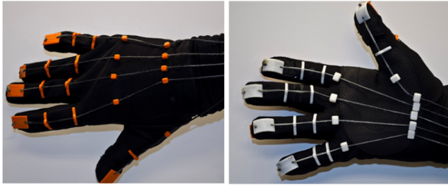
Figure 4: Cable guide assembly on glove. Cable lines run centered down the middle of the long axis of each digit and are attached rigidly at the fingertips. Note fingertip, phalanx, and palmar guides.
