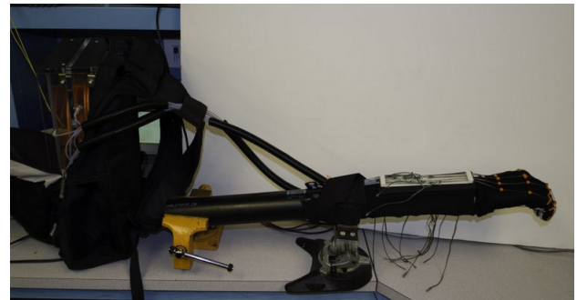
Figure 11: Wooden mannequin grip verification test. The glove is equipped on a wooden hand with pin-jointed fingers. The servomotors were actuated to their open and close hand positions and the mannequin hand was flexed and extended.
