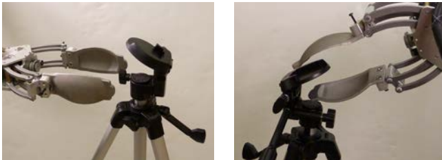
Fig. 5: The gripper in the desired preshaping configurations for grasping the tilt release knob and the mounting plate of the tripod
