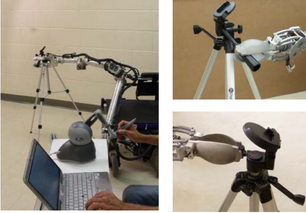
Fig. 4: Test-bed consisting of the master device, the robotic arm with gripper mounted on it and the object to be grasped
