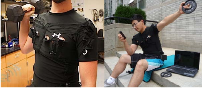
Fig. 2. Healthy human subjects wearing the sensorized shirt during weight lifting exercises.
