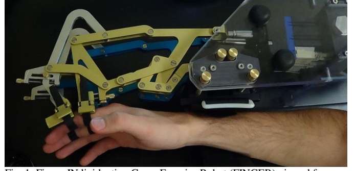
Fig. 1. Finger INdivuating Grasp Exercise Robot (FINGER) viewed from the top. FINGER can individually guide the index and pointer fingers through a naturalistic grasping motion.
