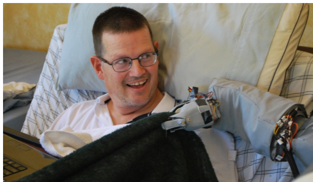
Fig. 1: Henry Evans, a person with quadriplegia, pulls a blanket over himself while in bed at home using our robotic system with whole-arm tactile sensing. As shown, the robot’s forearm made contact with his body and the bed.
