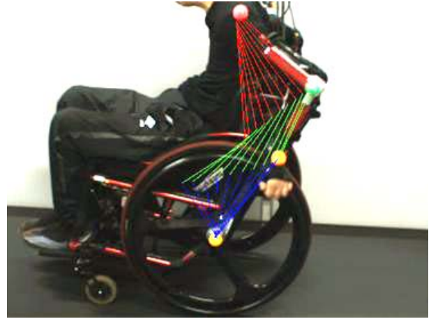
Fig. 4. Experimental setup of motion assistance for wheelchair operation with wearable robot by the individual with C5-level CCI (1.0[km/h], 7.0[%])
