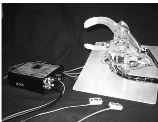
Fig. 2. AIST 3-DOF prosthetic hand, controller, and myoelectric sensors
