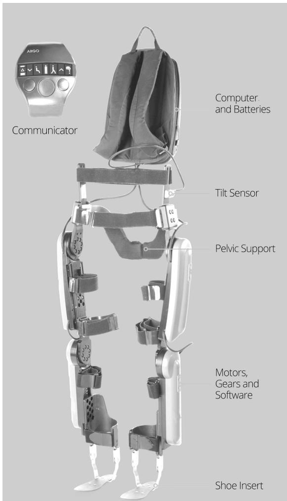
Fig. 1. The basic configuration of the ReWalk device.
