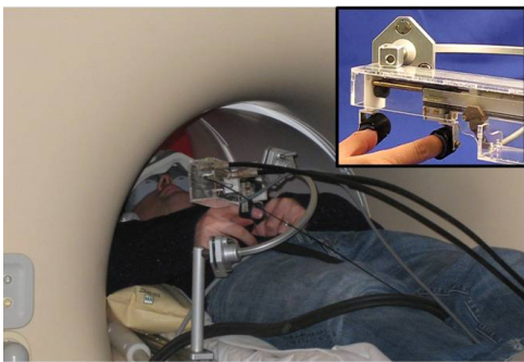
Fig. 1. Experimental setup. The forefinger manipulator was anchored to the scanner bed via an adjustable mount. In the inset, a close-up of the manipulator is shown.
