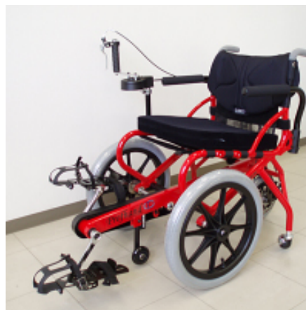
Fig. 1 Cycling wheelchair “Profhand” (TESS Co., Ltd.) developed by our research group in Japan.
