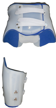
Fig. 7. Pelvis and thigh interfaces. These parts were molded on a subject by an orthopaedic technician.
